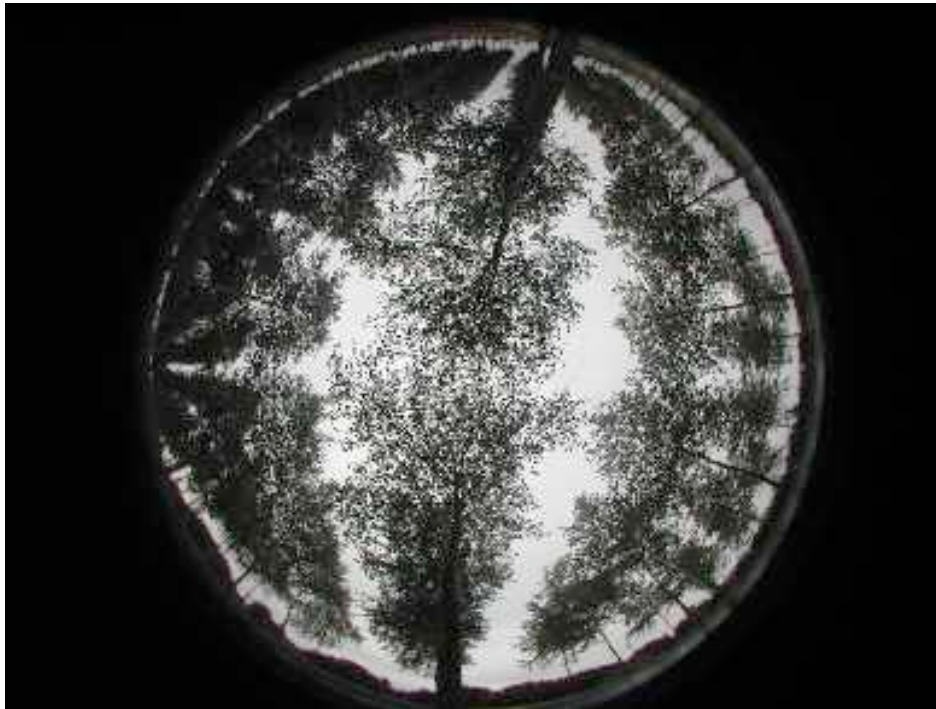
Fig 10. Example of a hemi-spherical photograph taken below an eleven-year-old widely-spaced poplar plantation (10 m x 6.4 m spacing)
